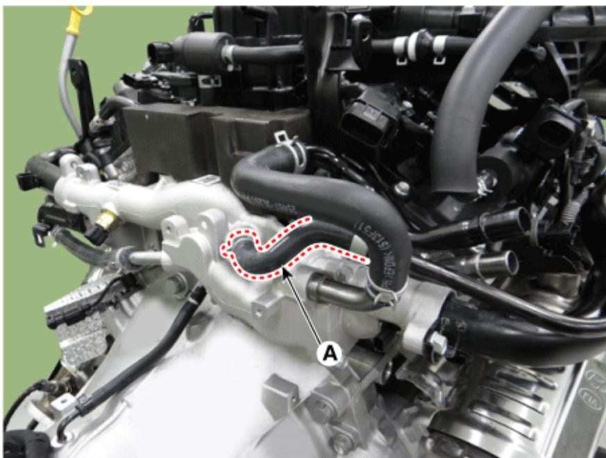
5. Disconnect the electric throttle control (ETC) module water hose (A).
