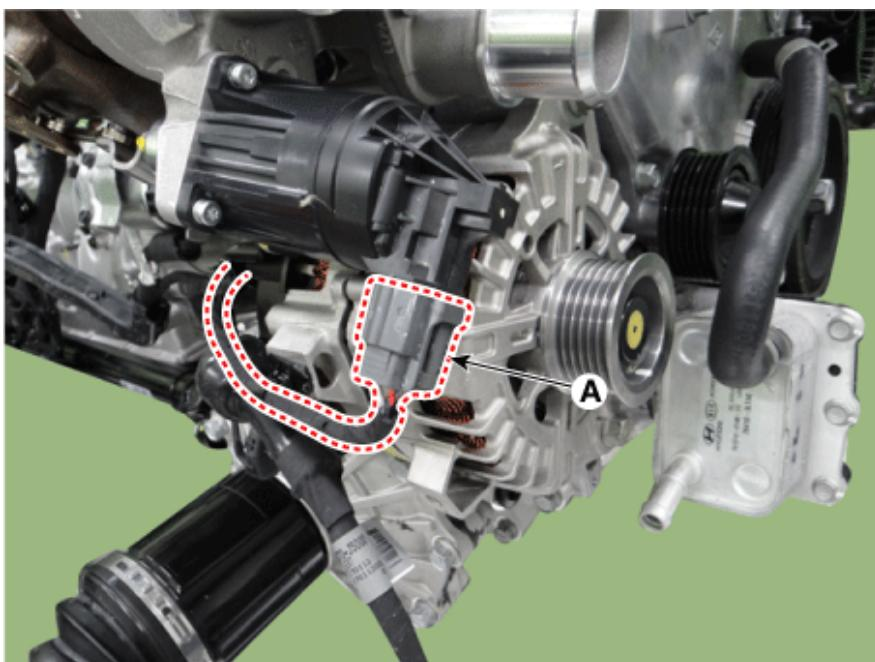
3. Remove the RH turbo manifold module heat protector (A).
