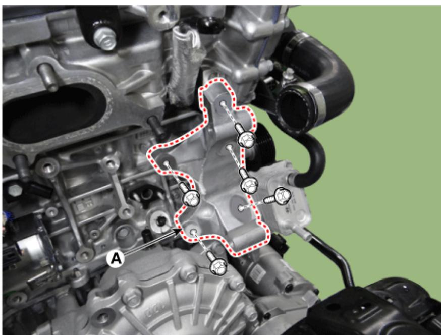
26. Remove the RH turbocharger oil feed pipe (A).
