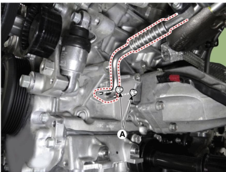
15. Remove the LH turbo manifold module stay (A).
