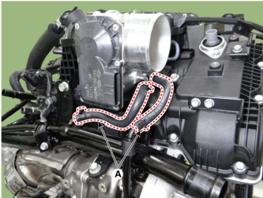
6. Disconnect the oil cooler water hose B (A).
