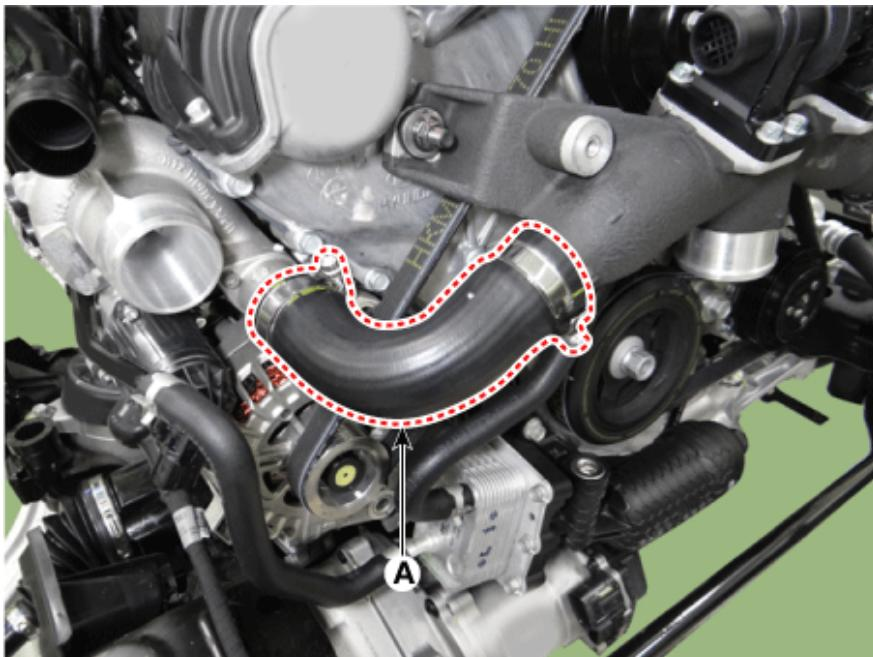
10. Remove the RH warm-up catalytic converter (WCC) stay (A).
