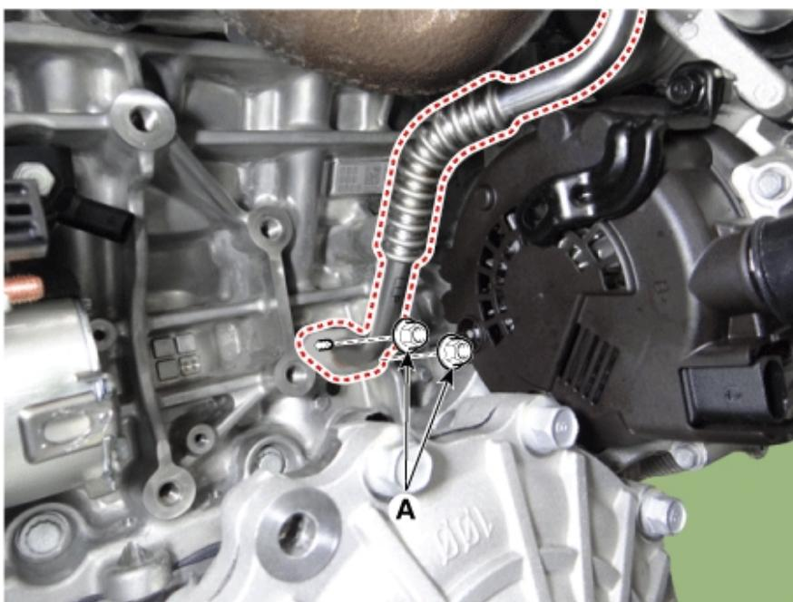
19. Remove the RH turbo manifold module stay (A).
