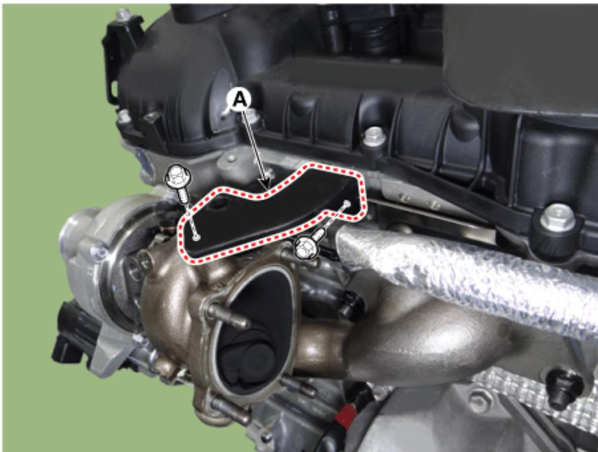
16. Remove the LH turbocharger oil feed pipe (A).
