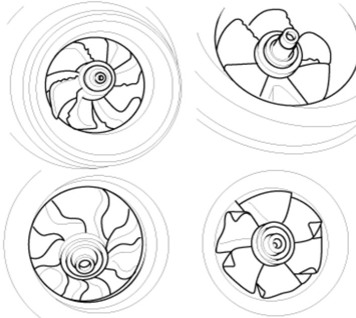
If the compressor wheel are damaged, it may cause abnormal noise from the turbocharger and poor acceleration.
