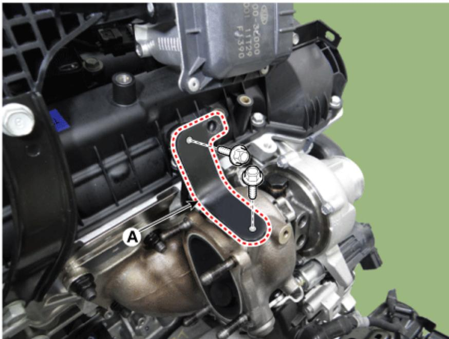
20. Remove the RH turbocharger oil feed pipe eye bolt (A).
