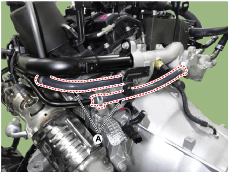
5. Remove the LH turbocharger water hose & pipe (A)
