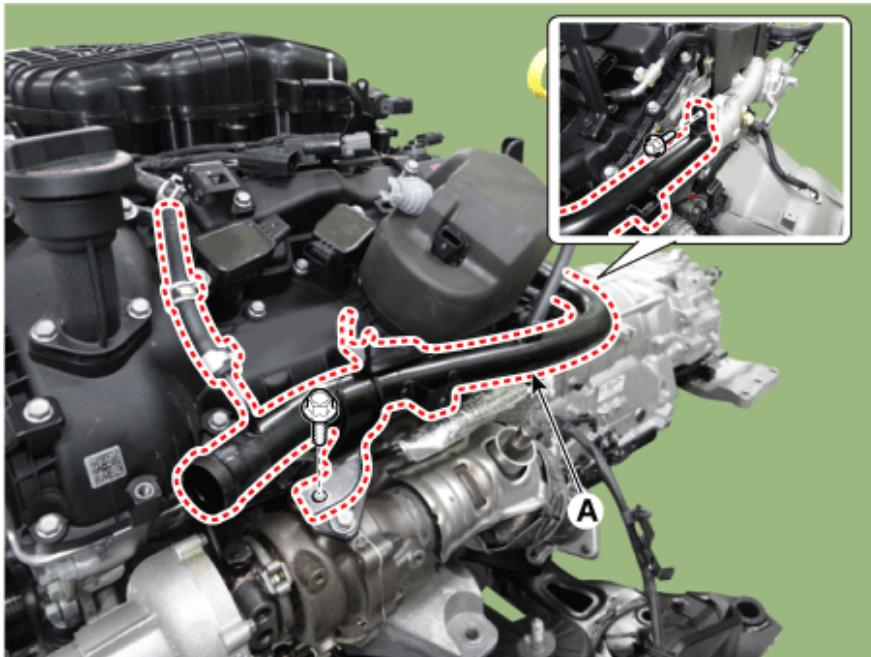
9. Disconnect the LH intercooler inlet hose (A).
