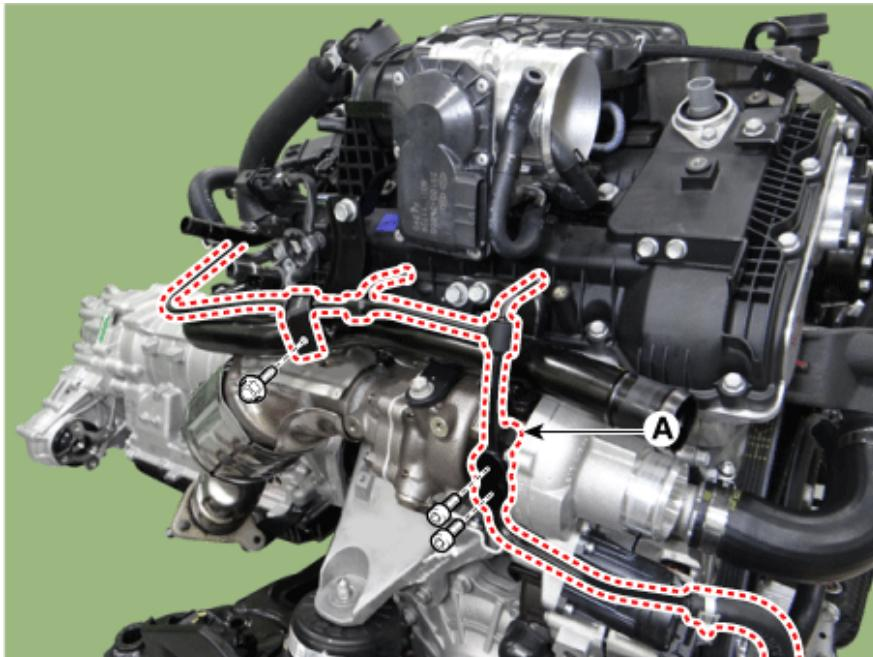
8. Remove the water inlet pipe (A).
