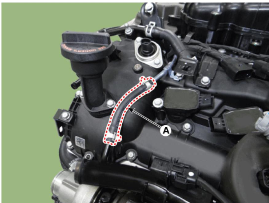
8. Remove the water outlet pipe (A).
