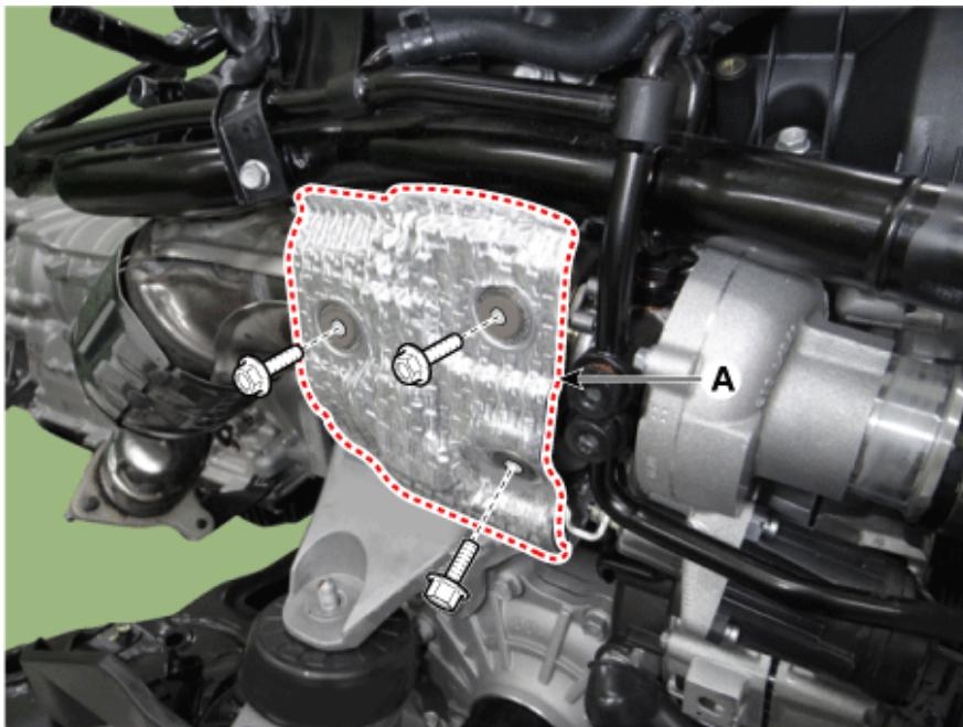
4. Disconnect the RH turbocharger water hose (A).
