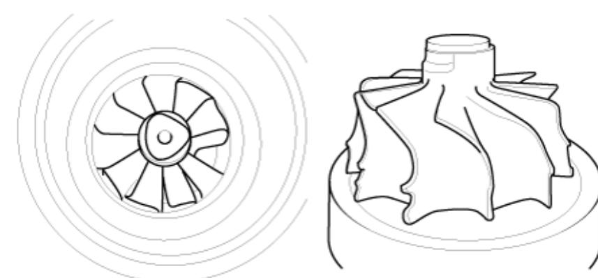
If the turbine wheel are damaged, it may cause abnormal noise from the turbocharger and poor acceleration.
