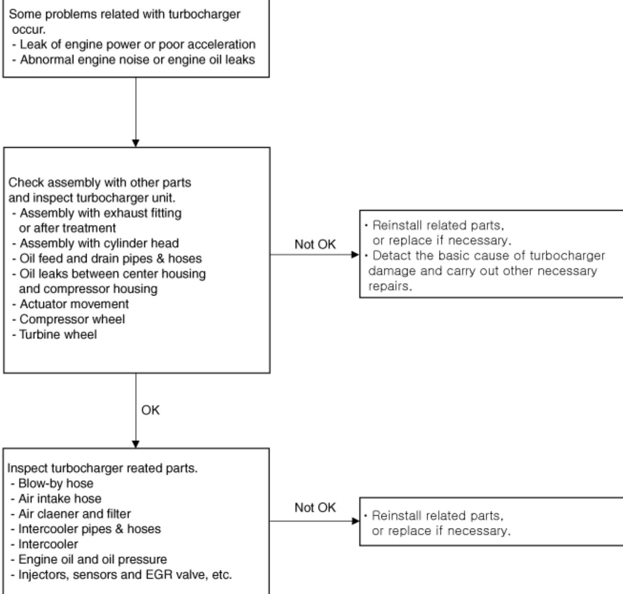
If any problem related with turbocharger, such as lack of engine power, poor acceleration, abnormal engine noise or oil leaks, may occur, check the turbocharger according to the procedure as follows.
