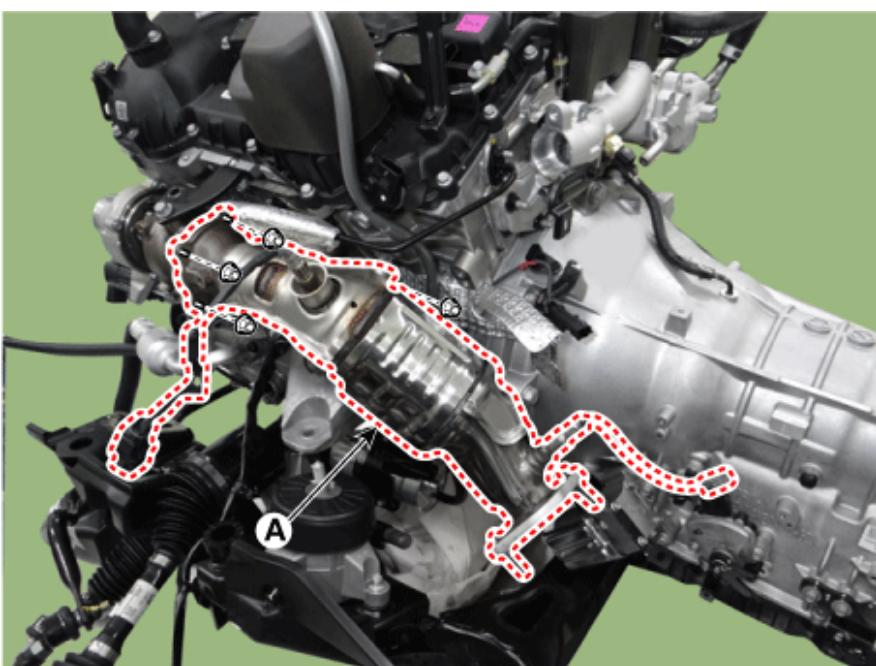
12. Remove the LH warm-up catalytic converter (WCC) gasket (A).
