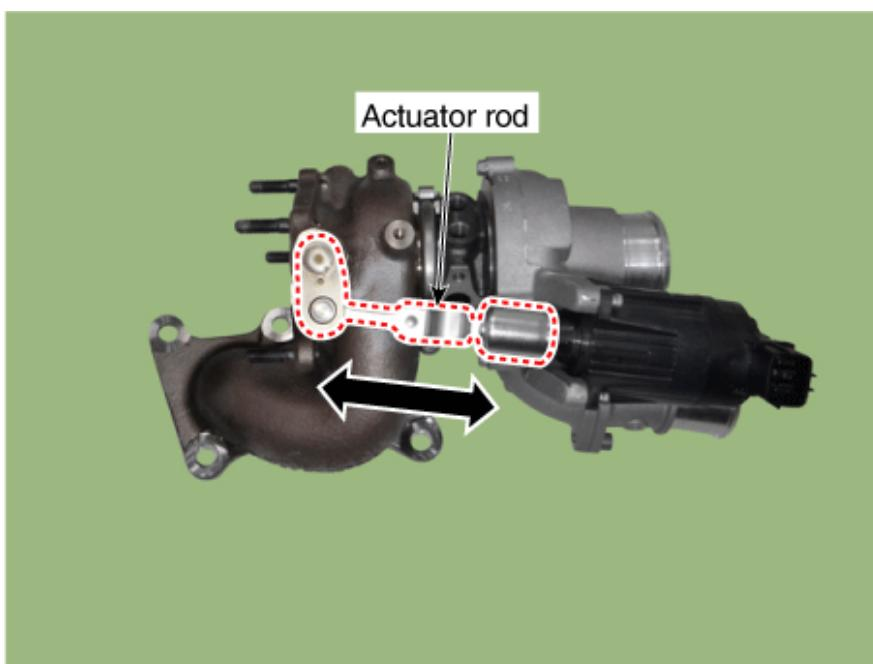
If the turbocharger actuator is damaged, it may cause lack of engine power and poor acceleration.
