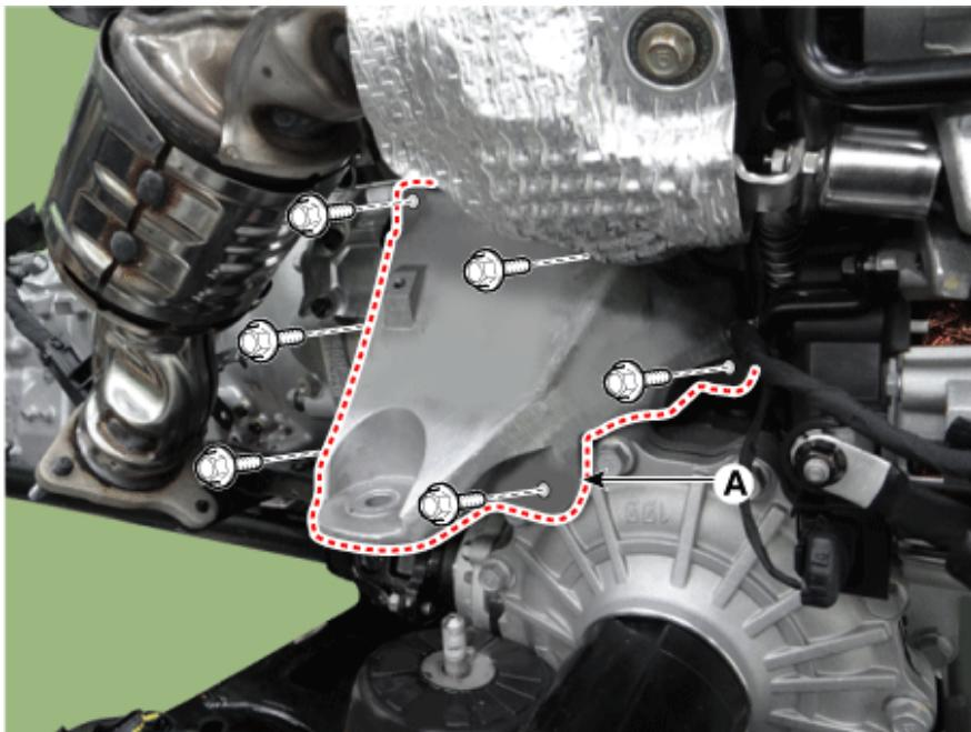
18. Remove the RH turbocharger oil drain pipe mounting nuts (A).
