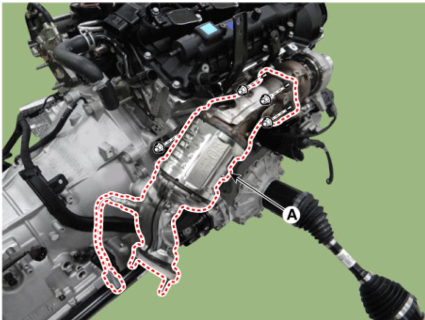
13. Remove the RH warm-up catalytic converter (WCC) gasket (A).
