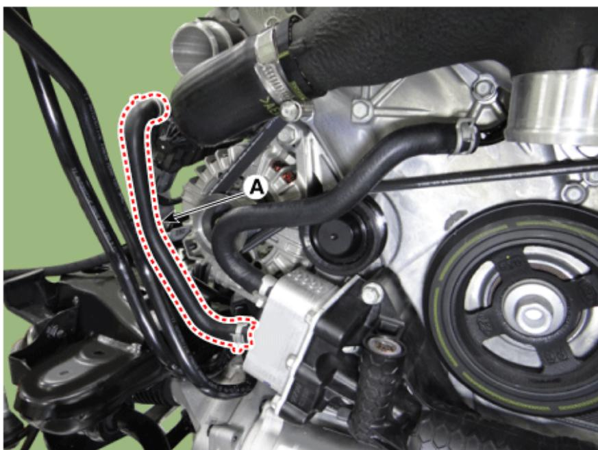
7. Remove the RH turbocharger water hose & pipe (A)
