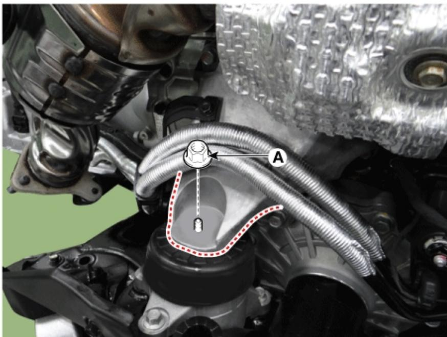
15. Hook the engine hoist to the hole of engine hanger.
