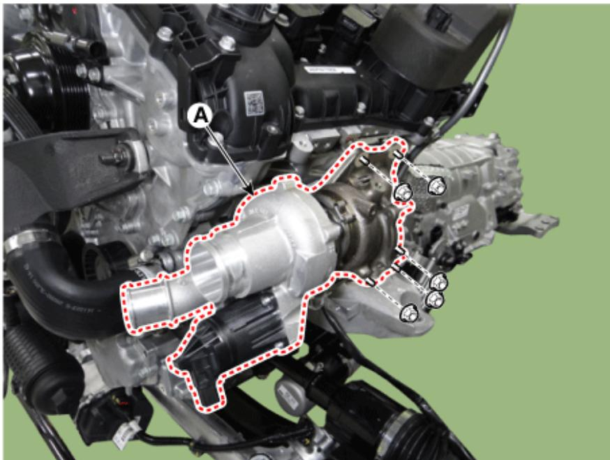
18. Remove the LH turbo manifold module gasket (A).
