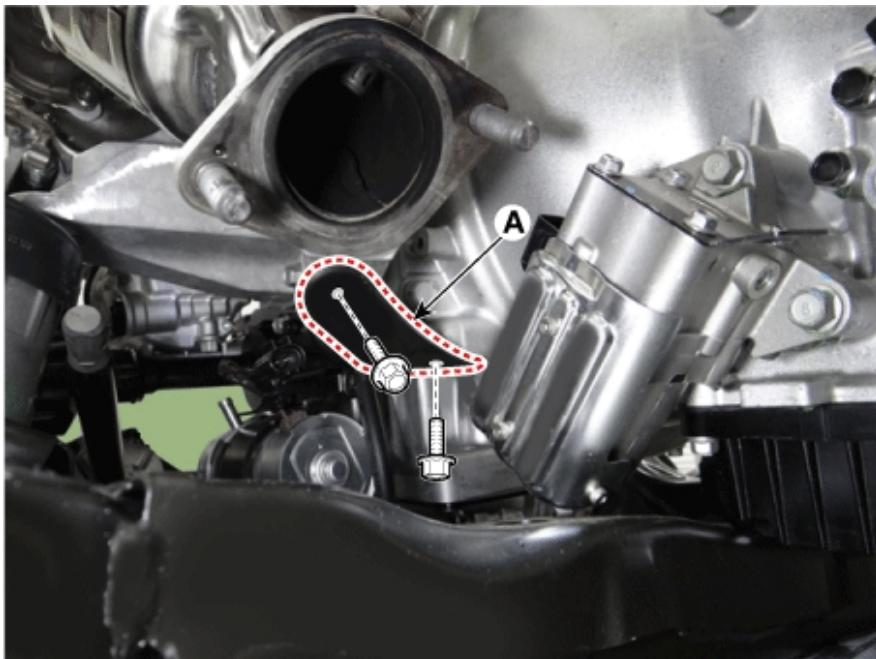
11. Remove the LH warm-up catalytic converter (WCC) (A).
